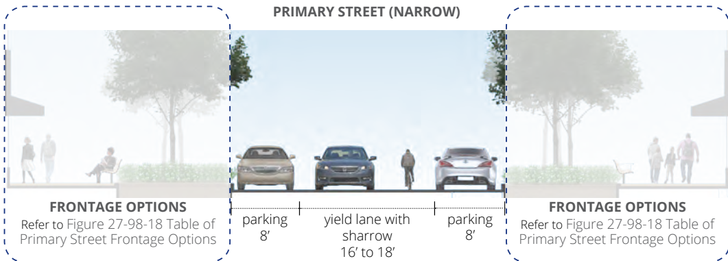
Figure 27-98-17 Primary Street Type Section: Narrow
