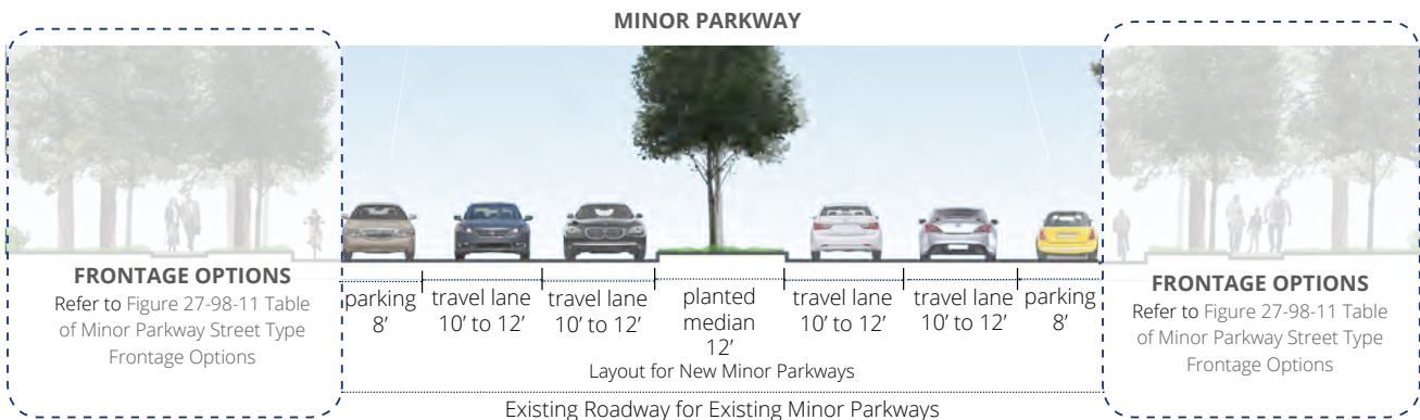
Figure 27-98-10 Minor Parkway Street Section - Existing and New
